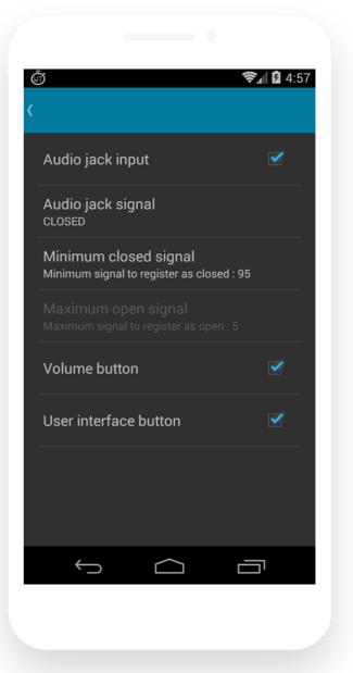
The Starter can be configured to accept either OPEN or CLOSED circuits. It listens to the microphone channel for a signal that exceeds the configured volume. The documentation for your Starting Pistol will provide the appropriate information. The one most commonly supported by Starting Pistols is CLOSED which is the default.
